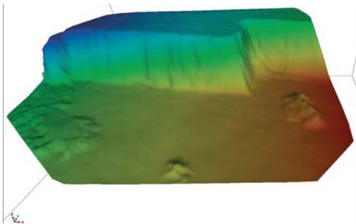
Figure 7. Laser scanner supported detection of the bench and the blasting system before blasting; The false colour plot is used to image the details of the bench morphology.
