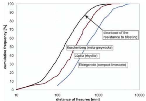
Figure 4. Cumulative curve of the three combined main joint directions for the metagreywacke (Koschenberg), rhyolite (Lueptitz) and limestone (Elbingerode) rock mass.
