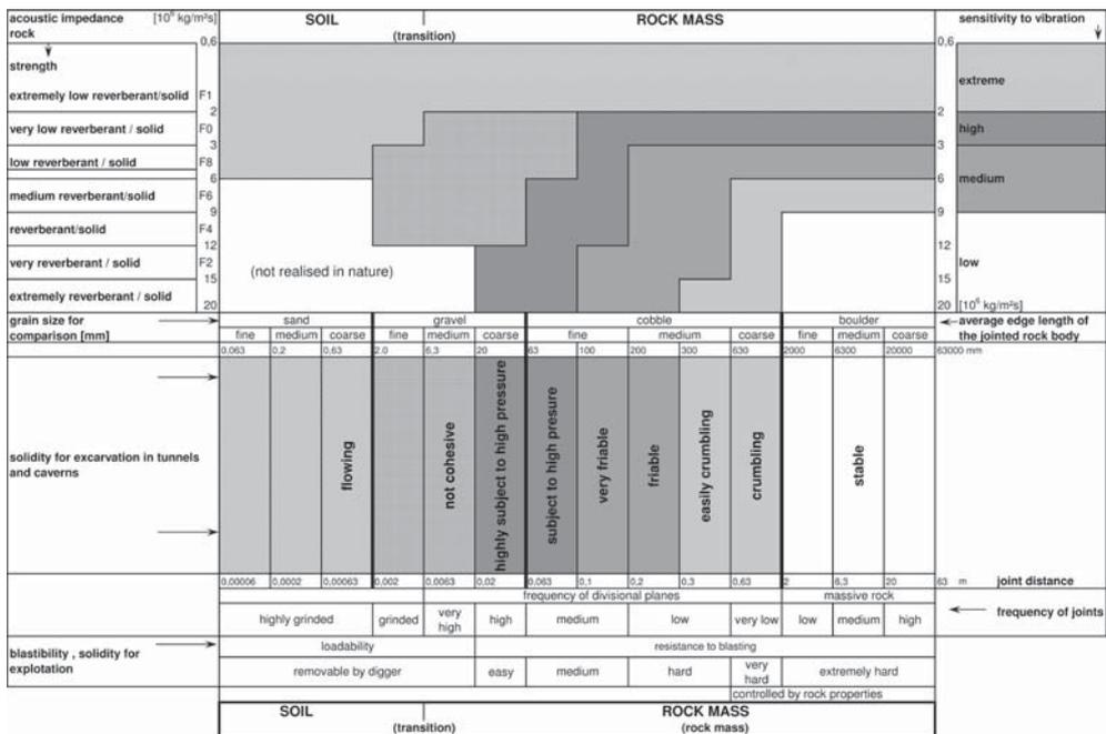
Figure 1. Rock mass and rock classification for rock and tunnel engineering and blasting technique (Müller 2007).
