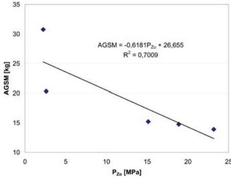
Figure 9. Correlation between the detonation pressure  $P_{zo}$  related to the unit volume ( $a_B \cdot w \cdot l_{B0}$ ) to the Average Grain Size Mass (AGSM), which is a product of the spherical volume of the representative grain size ( $d = 63.2\%$ ) in the cumulative curve and the rock density for various muck piles of blasted limestone.
