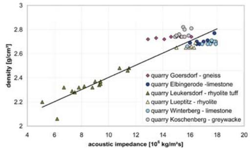
Figure 3. Correlation between the acoustic impedance and the rock density in the test quarries—initial rock parameters for resistance to blasting/blastability (see Figure 1).
