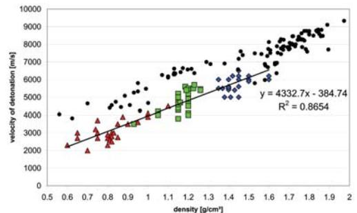
Figure 13. Coherencies between the explosive density and the detonation velocity of commercial explosives (data by Cooper 1996, Heinze 1993, Persson et al. 1994 and own measurements).
