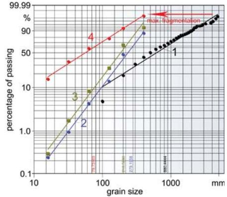
Figure 10. Comparison of grain size distributions of a rock mass (1) and some blastings (2–4) in the Rosin-Rammler-Sperling-Bennet-diagram (RRSB) for one quarry; one single hole fired blast (2) and two blastings with ignition system according to the momentum theory (3, 4).
