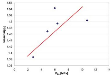
Figure 12. Influence to the muck pile loosening due to the value of detonation pressure per unit volume; the loosening can be defined as the proportion of the muck pile volume to the volume of the blast before firing.
