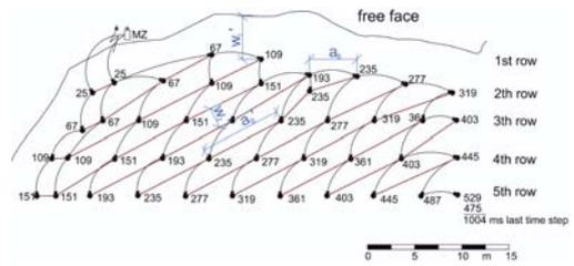
Figure 5. Drilling and ignition pattern of a test blasting with explanation;  $w'_{1/2}$ —blasted burden of the 1st row and the other rows (= blasted row distance  $a'_R = W'_2$ ) (Fischer et al. 2006).
