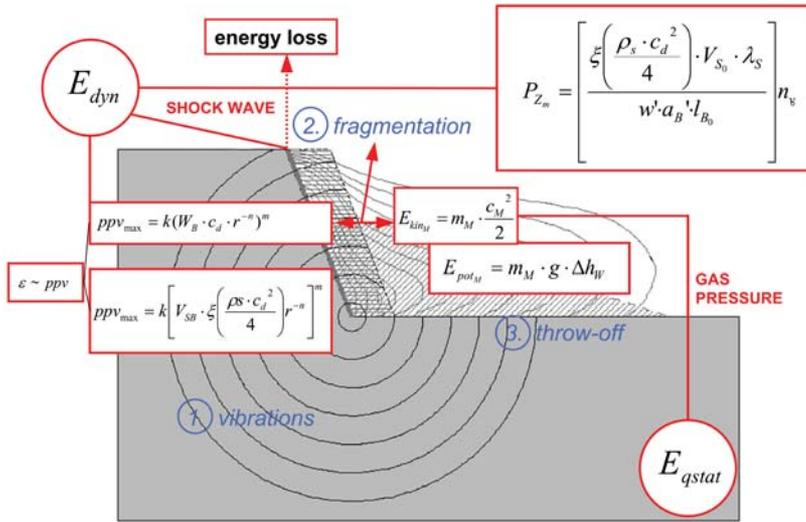
Figure 2. Physical effect model of a detonative reaction of explosives in a rock mass.
