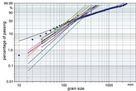
Figure 11. Exemplary analysis in the Rosin-Rammler-Sperling-Bennet-diagram (RRSB) of all muck pile distribution curves of various blasts of the quarry Koschenberg in comparison to the grain size distribution of the natural rock mass (dots).
