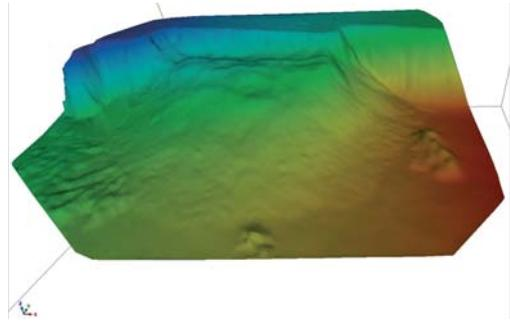
Figure 8. Laser scanner supported detection of the muck pile volume, the loosening and the new created bench; The false colour plot is used to image the details of the bench morphology.
