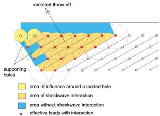
Figure 6. Principle of shockwave superpositioning during simultaneous ignition of charges according to the momentum theory.
